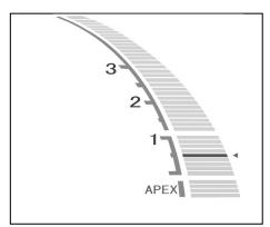
5. Check that all the meter indicator bars on the display are lit, the word "APEX" flashes and audible beep becomes continuous.
