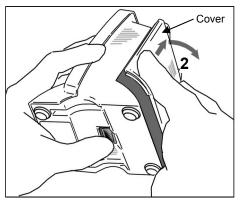
2. Slide the cover in the direction indicated by the arrow in the diagram to take it off.
