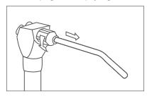
1. Unscrew and remove existing nut and tip. If nut, tip and adapter are screwed together, skip step 2.
