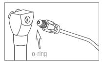
3. Verify that small o-ring is in the end of tip-adapter assembly. Screw assembly into syringe and finger tighten. Remove tip.
