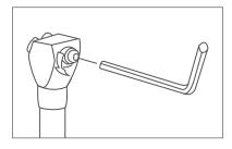
2. Unscrew and remove adapter using Allen Key. Some adapters may require a screwdriver to remove.
