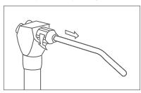
1. Unscrew and remove existing nut and tip.
