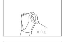
2. Verify that small o-ring is positioned inside the syringe at the back of the threaded opening. If not, use o-ring enclosed as replacement.
