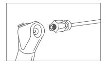
3. Screw tip adapter assembly into syringe. Tighten firmly.
