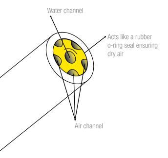
Seal-Tight features an inner yellow rubber seal that acts like a new o-ring with each tip replacement. This ensures dry air with every use.
