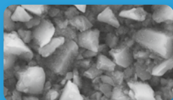
Venus One, Kulzer (1 \mu\text{m} ; 20,000x magnification)
