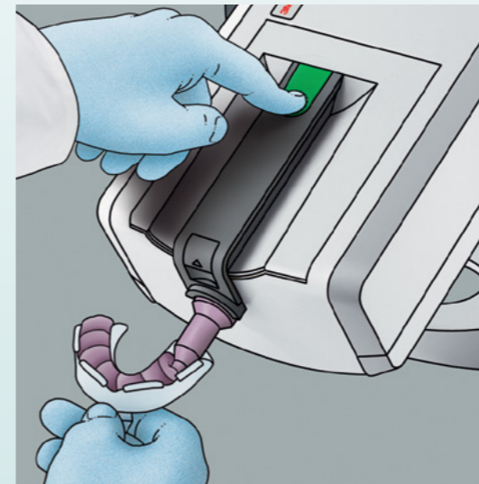
7. Press the green start button to fill the impression tray or elastomer syringe.
