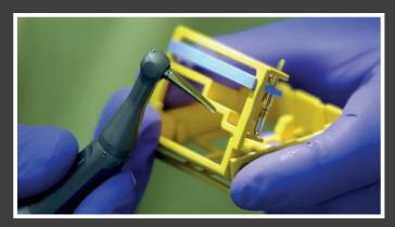
Insert the Periotome Tip into the handpiece, starting with 2mm tip.
